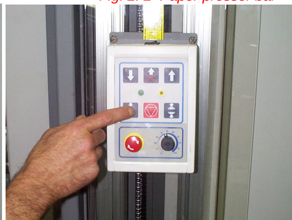
Fig. 2. 2 Paper presser bar
